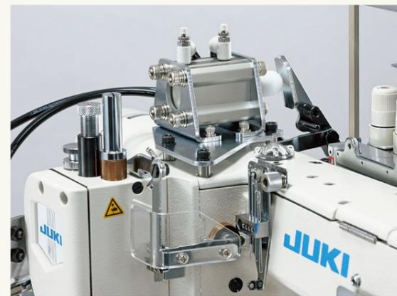
The presser foot can be lifted/lowered by depressing the back part of the pedal. This helps reduce operator fatigue, as lifting/lowering of the presser foot is frequently carried out during sewing work.
