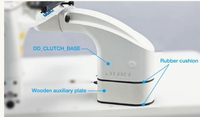
The MT-05 (DD\_CLUTCH\_BASE asm) is required to install the belt-drive type sewing machine on the table.
